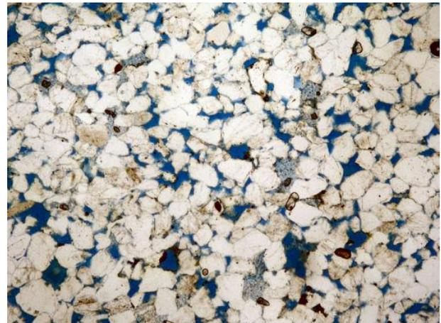
**Figures 3 & 4:** Photomicrographs of Craigleith sandstone, as it appears in thin section. The images were taken in plane-polarised light, and the field of view is c. 3.3 mm. Pore space appears blue.
