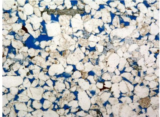
**Figures 1 & 2:** Photomicrographs of Hazeldene sandstone, as it appears in thin section. The images were taken in plane-polarised light, and the field of view is c. 3.3 mm. Pore space appears blue.
